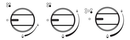
Fig. 14a Burner knob and symbols (CG604 models (no flame failure))
